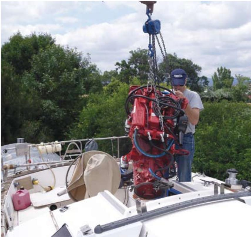
with its accessories. This provided exact positioning of the vibration mounts and the driveshaft and did not require the shop crane to move around. The mockup was invaluable, as it exposed the fact that the engine bed had to be lowered by 3 1/4". As it turns out, the old engine mounts were not on the plane of the crankshaft, but rather were vertically offset to lower the engine. I had missed this detail when specifying the engine.
