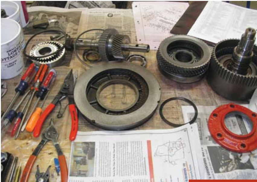
From the top: the fully deconstructed transmission, freshly repainted case parts and shiny new clutch disks. Opposite: the all-important owner's manual
